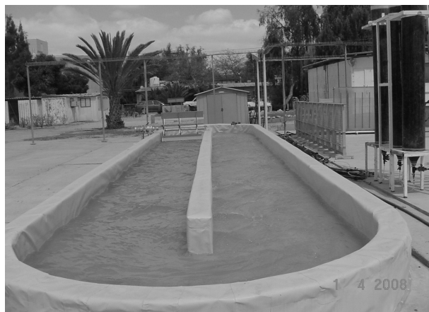
Figure 3. A typical open pond driven by a simple paddle wheel for the cultivation of an alga. With kind permission of Professor S. Boussiba, Ben Gurion University of the Negev, Israel; (a colour photograph of this figure is available on: http://bidr.bgu.ac.il/bidr/research/algal/Facilities.htm ).
