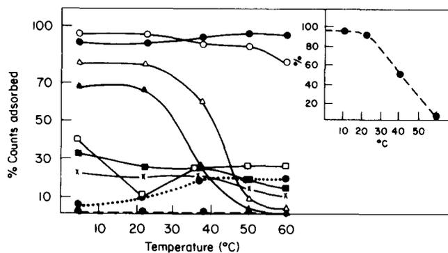
**Figure 3.** Temperature effect. Adsorption of  $^3\text{H}$ -poly(A) to different matrices as a function of temperature. The columns were calibrated with 0.4 M NaCl in 10 mM Tris HCl buffer, pH 7.6, in a temperature chamber. The percent radioactivity adsorbed with respect to the total amount of material is plotted. Symbols as in Figure 1
