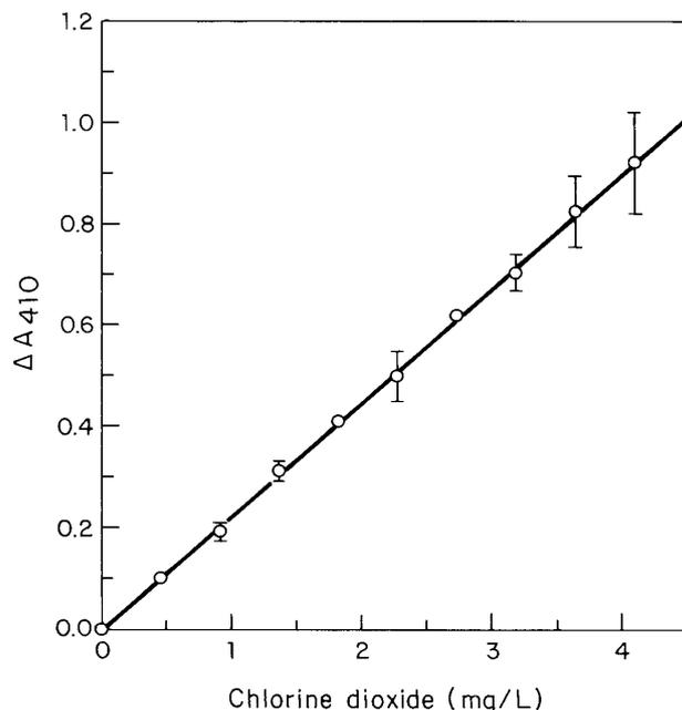
FIG. 4. Calibration curve for chlorine dioxide determination by the biochemical method. The reaction mixture contained  $50 \mu\text{g/ml}$  of reactive yellow 17 and  $0.8 \text{ nmol/ml}$  of horseradish peroxidase.  $\Delta A_{410}$  was obtained after a 15-min reaction.
