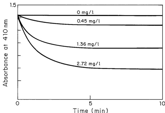
FIG. 2. Reaction kinetics of reactive yellow dye with different concentrations of chlorine dioxide. The reaction mixture contained 50  $\mu\text{g/ml}$  of dye and 0.8 nmol/ml peroxidase.
