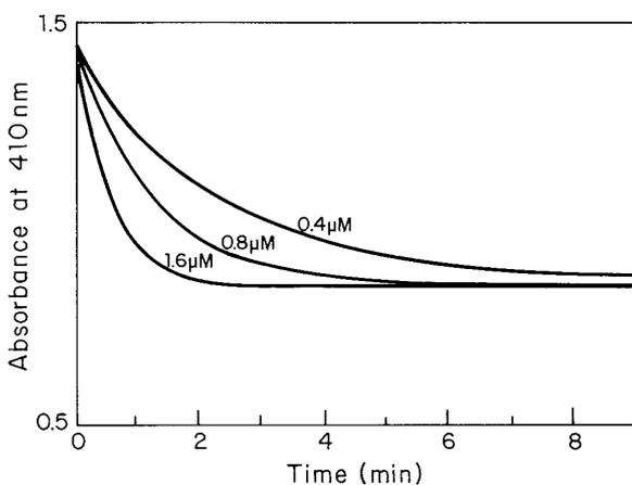
FIG. 1. Reaction kinetics of reactive yellow dye with different amounts of horseradish peroxidase. The reaction mixture contained 50  $\mu\text{g/ml}$  of dye and 2.8  $\mu\text{g/ml}$  chlorine dioxide.
