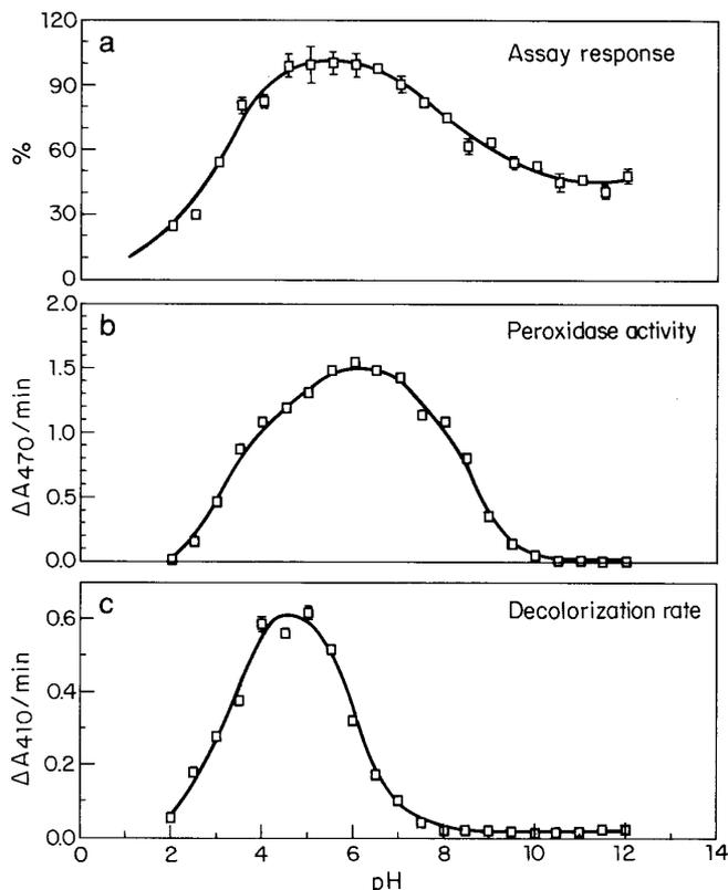
FIG. 3. The effect of pH on (a) chlorine dioxide determination by the biochemical method, (b) decolorization rate of reactive yellow in the presence of horseradish peroxidase and  $\text{ClO}_2$ , and (c) peroxidase activity as guaiacol oxidation in the presence of hydrogen peroxide. The buffer solutions used were 60 mM sodium acetate for pH 2–5, 60 mM sodium phosphate for pH 5.5–7.5, and 60 mM sodium bicarbonate for pH 8–12.
