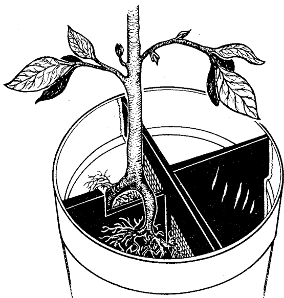
Fig. 1. Four-chambered growth container for the separation of Vesicular-arbuscular mycorrhizal (VAM) roots from VAM hyphae (by a 44- \mu\text{m} screen) on one side of a solid barrier, and non-VAM roots from control soil (screen) on the other.
