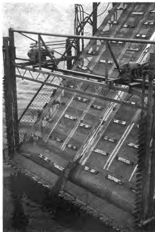
Figure 6. Cutters mounted on the front of a vessel for harvesting Macrocystis pyrifera . When harvesting, the reciprocating cutters and conveyor belt are lowered one metre below the surface and the cut seaweed is forced onto the belt by the forward motion of the vessel.
