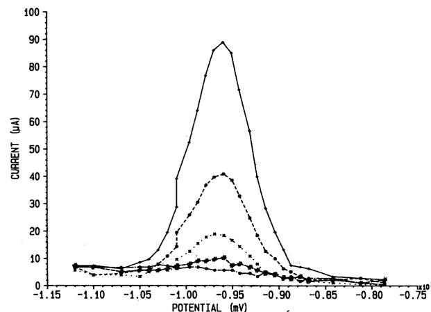
FIG. 3. ASV voltammogram of  $Zn^{2+}$  added to dissolved polysaccharide ( $45 \mu g$  of glucose equivalent  $ml^{-1}$ ) of *C. stigmatophora*. Symbols: ●, 0; #, 200; ×, 250; ■, 300; +, 400 ppb of  $Zn^{2+}$ .
