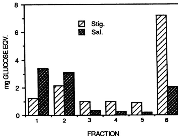
FIG. 6. Elution profile of the polysaccharide of *C. stigmatophora* and *C. salina* on a DE-52 anion exchange column. Fractions: 1, double-distilled water; 2, 0.5 M NaCl; 3, 1.0 M NaCl; 4, 2.0 M NaCl; 5, 5.0 M NaCl; 6, 6.0 M urea.
