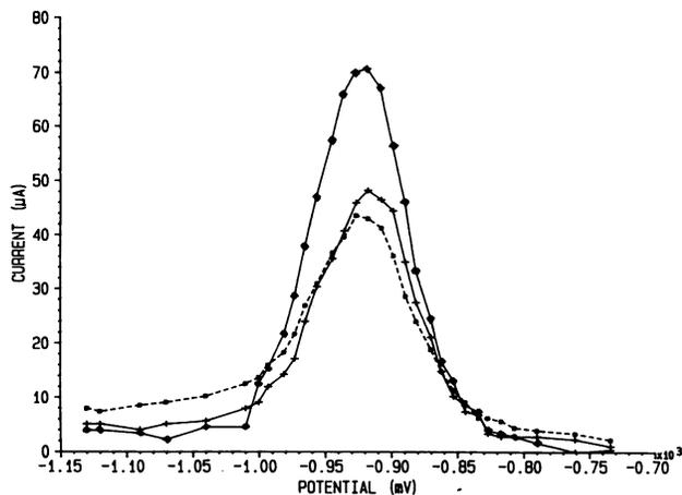
FIG. 4. ASV voltammogram of  $Zn^{2+}$  added to dissolved polysaccharide ( $48 \mu\text{g}$  of glucose equivalent  $\text{ml}^{-1}$ ) of *C. salina*. Symbols: ■, 0; +, 10; ♦, 80 ppb of  $Zn^{2+}$ .
