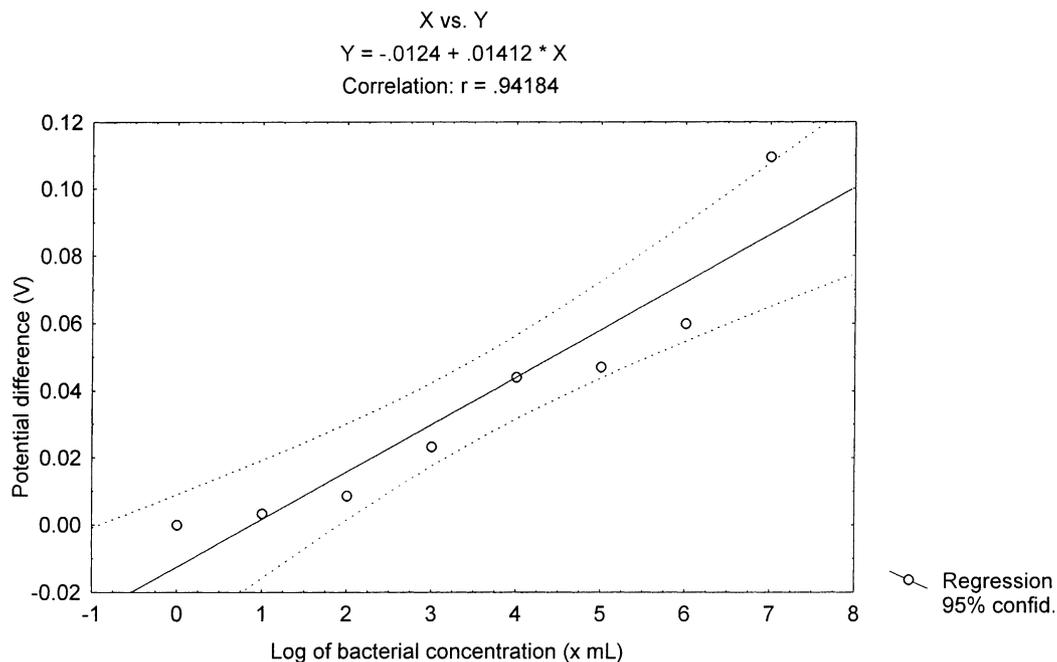
Fig. 4. Plot representing *E. coli* cell concentration vs. potential differences. The calculated LOD appears to be 7.5 bacteria per ml.
