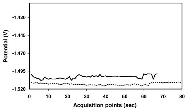
Fig. 5. Acquisition curves of *K. oxytoca* (top line) and *P. marina* (bottom line) in the presence of polyclonal *E. coli* antibodies. Cells were attenuated and diluted to  $10^6 \text{ ml}^{-1}$  for both *K. oxytoca* and *P. marina*.
