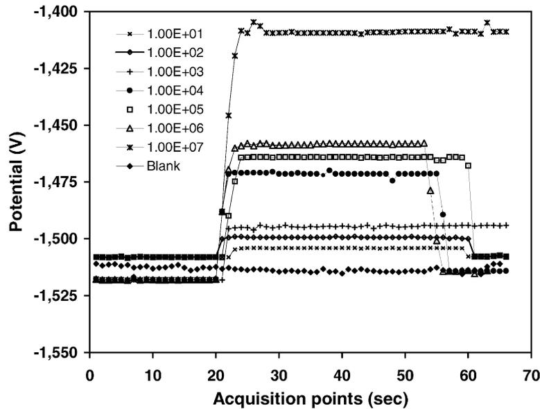
Fig. 3. Acquisition curves of different *E. coli* concentrations in the presence of polyclonal *E. coli* antibodies: the samples contained *E. coli* cells ranging from  $10$ – $10^7$   $\text{ml}^{-1}$ . Blank acquisition curve obtained by flowing urea on a cover slip treated as the samples but with cell-free is also reported.
