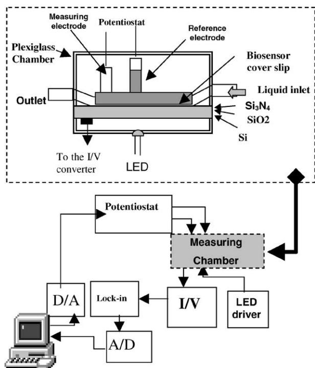
Fig. 1. Block diagram of the transducer system. On top a detailed drawing of the measuring chamber is reported with the sensing electrode made of silicon, silicon dioxide and silicon nitride. In the bottom, the signal measurements performed by a synchronous demodulation techniques and the conditioning electronics blocks are shown.
