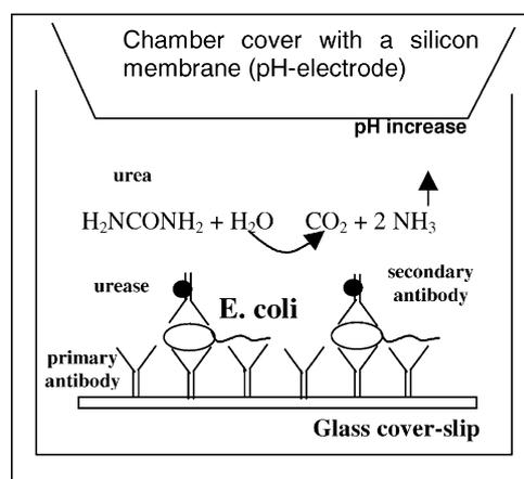
Fig. 2. Biological component of the sensor. The primary anti-*E. coli* antibody is coated on a silanised glass cover slip. *E. coli* present in the sample link to the antibody and the secondary urease-bound antibody is fluxed and then washed with PBS. At the end urea is fluxed and the reaction is recorded.
