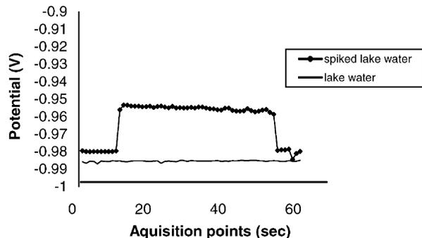
Fig. 7. Acquisition curves of water samples from the Lake of Bracciano (Rome) both untreated (bottom line), and spiked (top line) with  $1 \times 10^3$  *E. coli* cells per ml.
