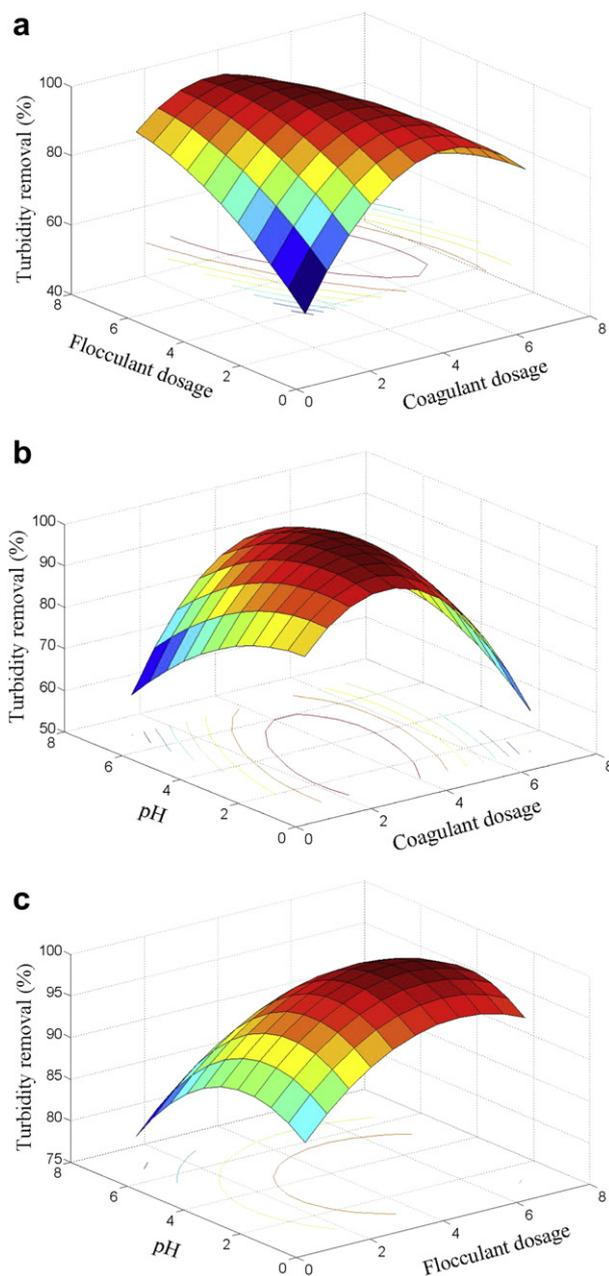
**Fig. 4 – 3D surface graphs and contour plots of turbidity removal efficiency showing the effect of variables: (a)  $X_1$ – $X_2$ ; (b)  $X_1$ – $X_3$ ; and (c)  $X_2$ – $X_3$ .**
