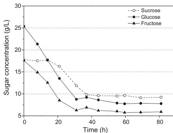
**Fig. 5.** The degradation profiles of the mixed sugars (sucrose, glucose and fructose) in tropical maize stalk juice during ABE fermentation.
