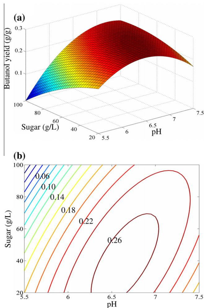
**Fig. 1.** Response surface and contour plots for butanol yield: effects of pH and sugar concentration (agitation rate was fixed at 48 rpm).
