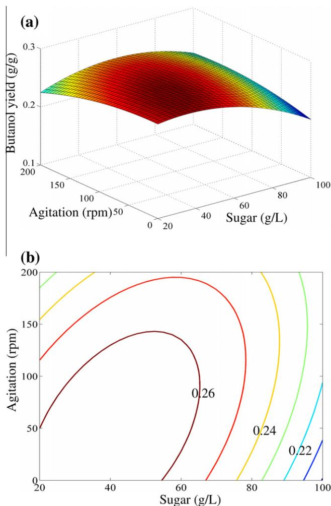
Fig. 3. Response surface and contour plots for butanol yield: effects of sugar concentration and agitation rate (pH was fixed at 6.7).
