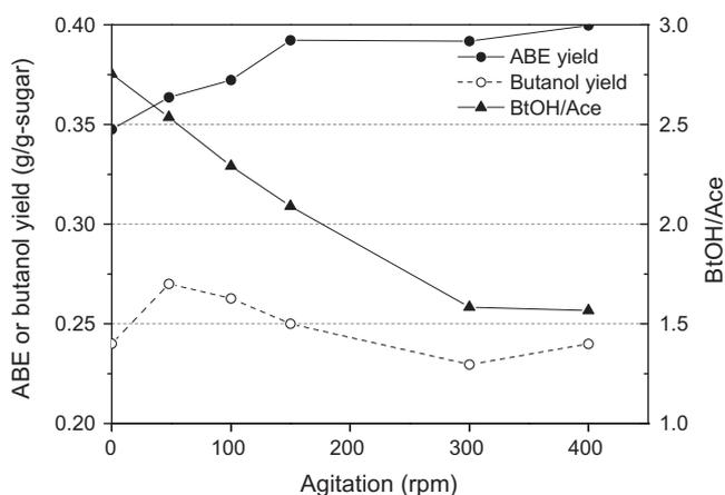
**Fig. 4.** The effect of agitation on final ABE yield, butanol yield and butanol/acetone (BtOH/Ace in the figure) ratio.
