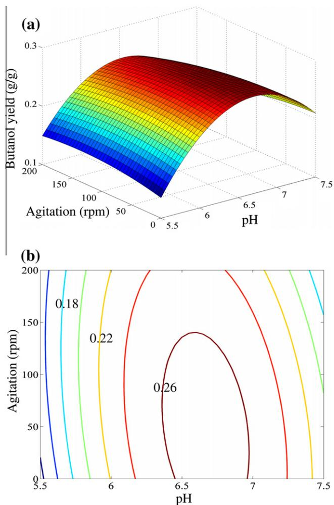
Fig. 2. Response surface and contour plots for butanol yield: effects of pH and agitation rate (sugar concentration was fixed at 42.2 g/L).
