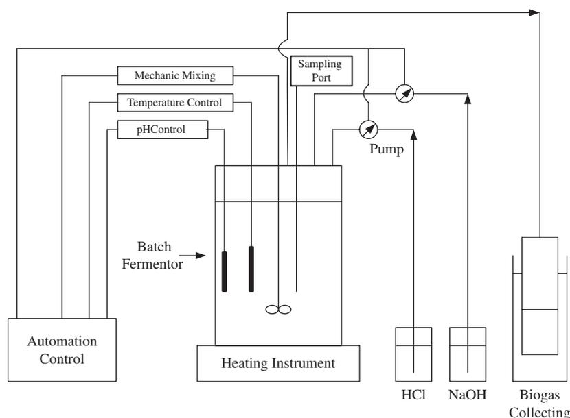
Fig. 1 – The schematic of the experimental setup.
