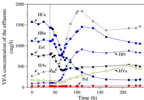
Fig. 3. Variation of aqueous products in the substrate shift (HAc = acetate; HPr = propionate; HBu = butyrate; HVa = valerate; HCa = caproate; Eol = ethanol; and Pol = propanol).
