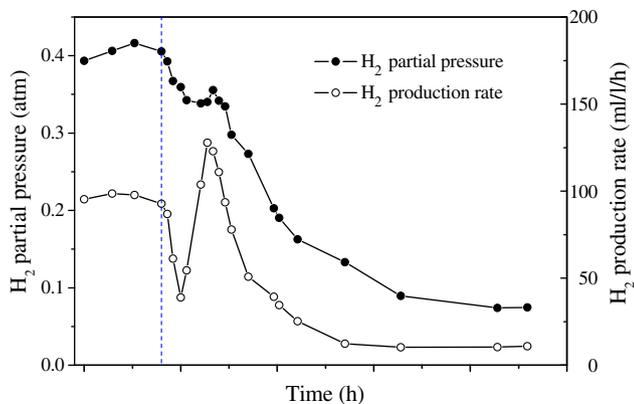
Fig. 2. Variation of H<sub>2</sub> partial pressure and H<sub>2</sub> production rate in the substrate shift.
