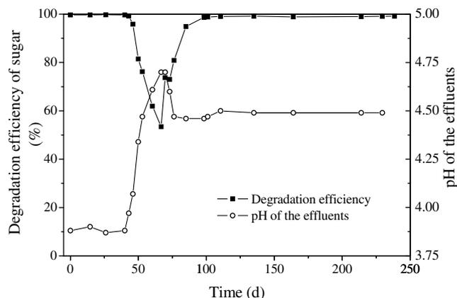
Fig. 1. Variation of substrate degradation efficiency and effluent pH in the substrate shift.
