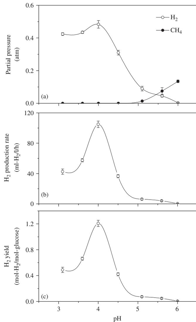
Fig. 4. Variation of: (a)  $H_2$  partial pressure in biogas, (b)  $H_2$  production rate and (c)  $H_2$  yield at various pHs in R2.
