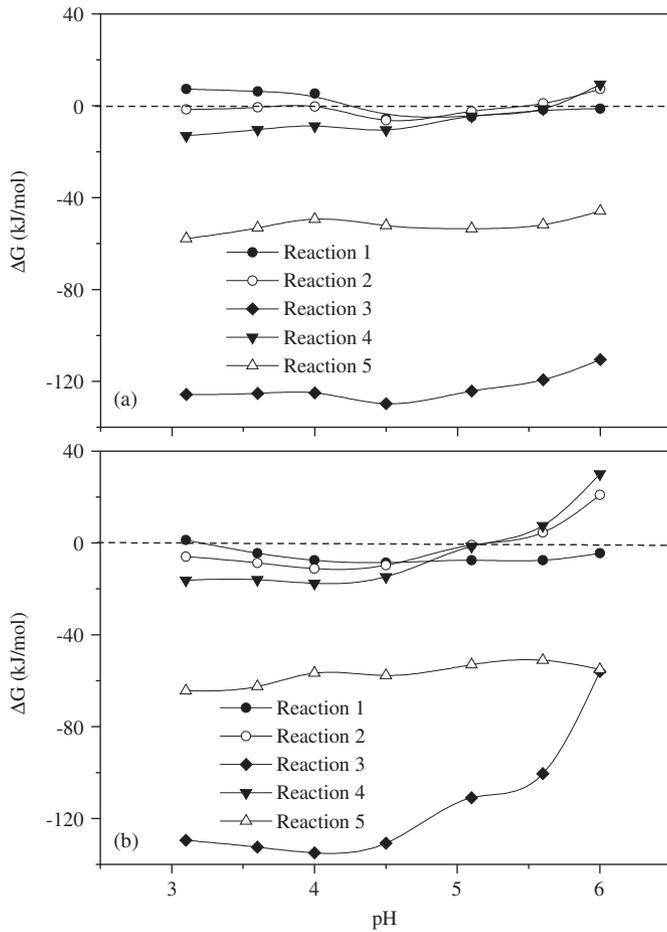
Fig. 5. Variation of Gibbs free energy for caproate formation at various pHs in: (a) R1; and (b) R2.
