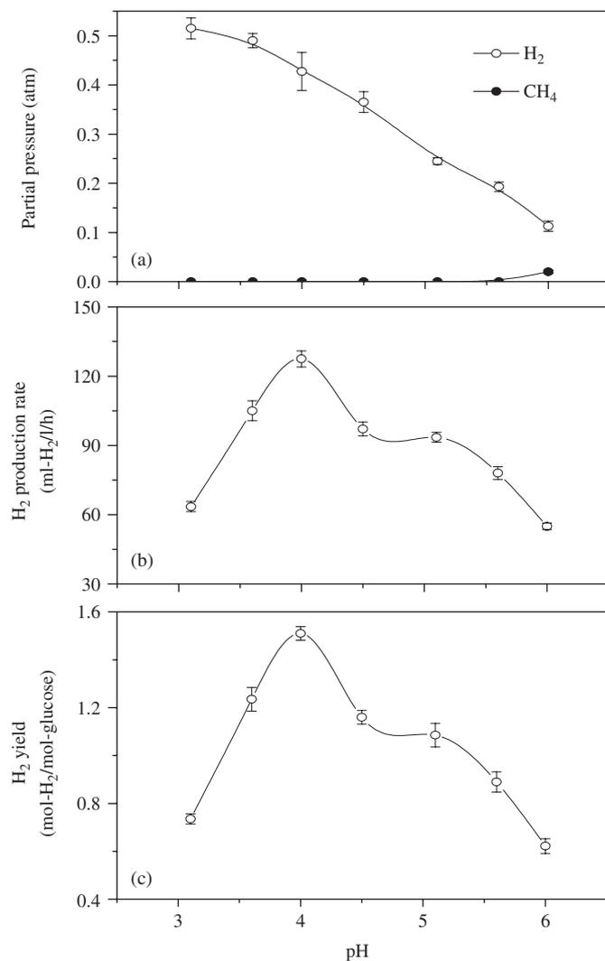
Fig. 3. Variation of: (a)  $H_2$  partial pressure in biogas, (b)  $H_2$  production rate and (c)  $H_2$  yield at various pHs in R1.
