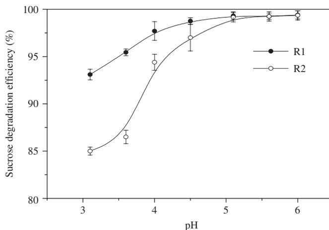
Fig. 2. Variation of substrate degradation at various pHs for R1 and R2.
