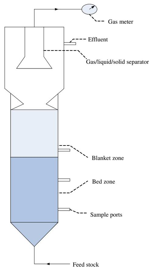
Fig. 1. Setup of the UASB reactors.
