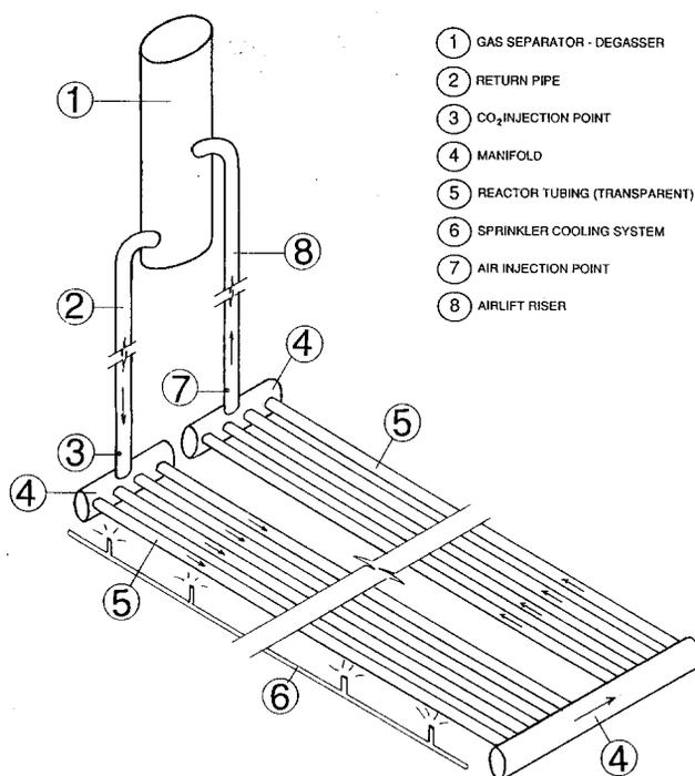
Fig. 1. Schematic diagram of the reactor (not to scale).
