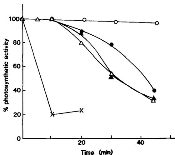
Fig. 5. The effect of temperature on the photosynthetic activity of *P. cruentum* cultures exposed to  $2300 \mu\text{mol photon m}^{-2} \text{s}^{-1}$  light. Chlorophyll concentration was  $13 \text{ mg chl.a}$ . (○)  $15^\circ\text{C}$ , (●)  $20^\circ\text{C}$ , (▲)  $25^\circ\text{C}$ , (△)  $30^\circ\text{C}$  and (×)  $35^\circ\text{C}$ . 100% activity corresponds to  $600 \mu\text{mol O}_2 \text{ h}^{-1} \text{mg}^{-1} \text{chl.a}$
