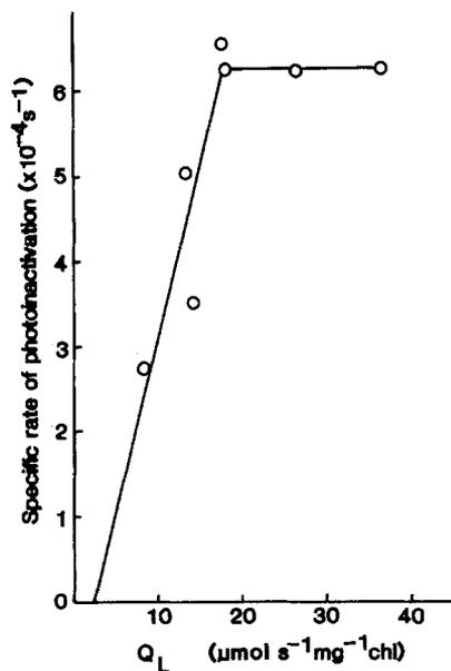
Fig. 4. Specific rate of photoinhibition of *P. cruentum* cultures vs. the specific light absorption rate. The specific rate of photoinhibition was calculated from the slope of the plot between  $\ln$  (Oxygen Production Rate) and the time of exposure to strong light
