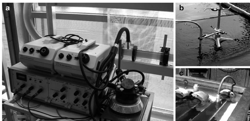
**Fig. 4** In-situ measurement of Chl fluorescence quenching using a fibre-optic guide and a pulse-amplitude-modulation fluorometer in a greenhouse tubular photobioreactor (**panel a**). The fibre-optics were protected in a glass test tube and submerged in
