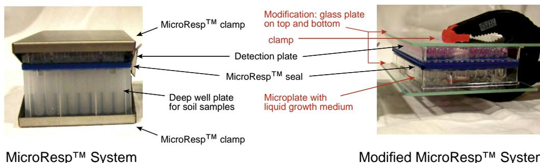
**Fig. 1.** Comparison of the original versus the modified MicroResp™ setup: the deep well plates for soil samples were replaced by microplates with liquid growth media containing a substrate or toxic chemical compound in microdilutions.
