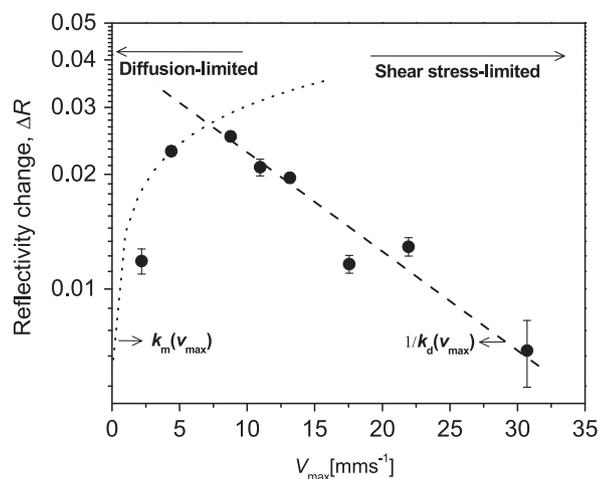
**Fig. 4.** Dependence of SPR sensor response  $\Delta R$  on the flow velocity  $v_{\max}$ . The concentration of *E. coli* K12 in PBST was of  $10^8$  cfu mL $^{-1}$  and the affinity binding to specific antibodies p-IgG on the surface probed by LRSPs.
