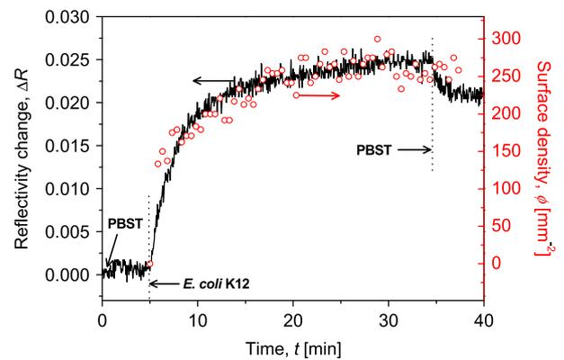
**Fig. 3.** Simultaneous observation of affinity binding of *Escherichia coli* K12 by SPR (sensor response  $\Delta R$ ) and optical microscopy (determined surface density). Analyte was dissolved in PBST at a concentration of  $10^8$  cfu mL $^{-1}$  and flowed with the flow velocity of  $v_{\text{max}} = 8.8$  mm s $^{-1}$ .
