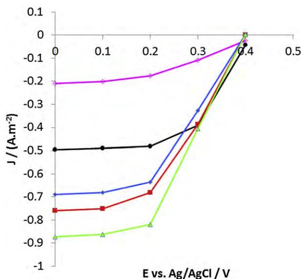
**Fig. 1.** Cathodic current density by surface (un)modified oxygen reducing biocathodes during polarisation (10 min equilibration time) after 20 days of operation. Green = unmodified; red = D-20; blue = D-0.5; black = N-20; magenta = N-0.5.
