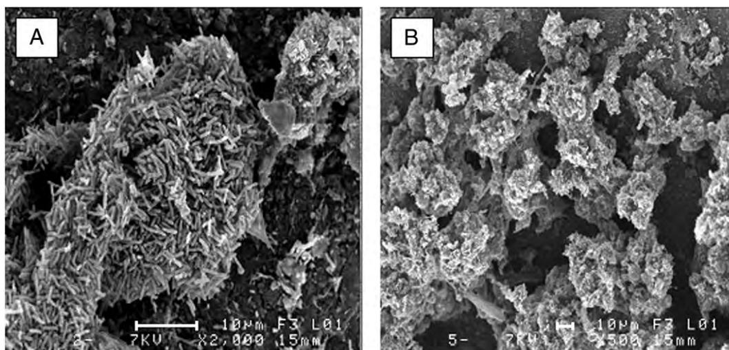
**Fig. 3.** Representative SEM pictures of oxygen reducing biofilms at biocathodes (A) a granule like cluster of microorganisms at the N-20 biocathode; (B) biofilm structure and coverage of the N-20 biocathode. Scale bar represents 10  $\mu\text{m}$ .
