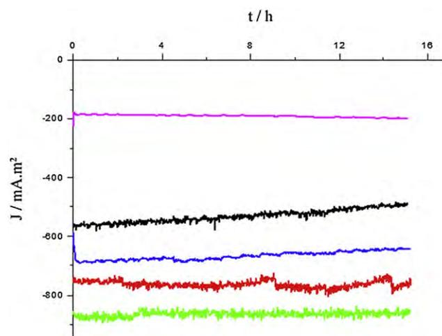
**Fig. 2.** Representative data of stable catalytic cathodic current densities at different oxygen reducing biocathodes operated at +0.150 V vs. Ag/AgCl after 20 days of operation. Green = unmodified; red = D-20; blue = D-0.5; black = N-20; magenta = N-0.5.
