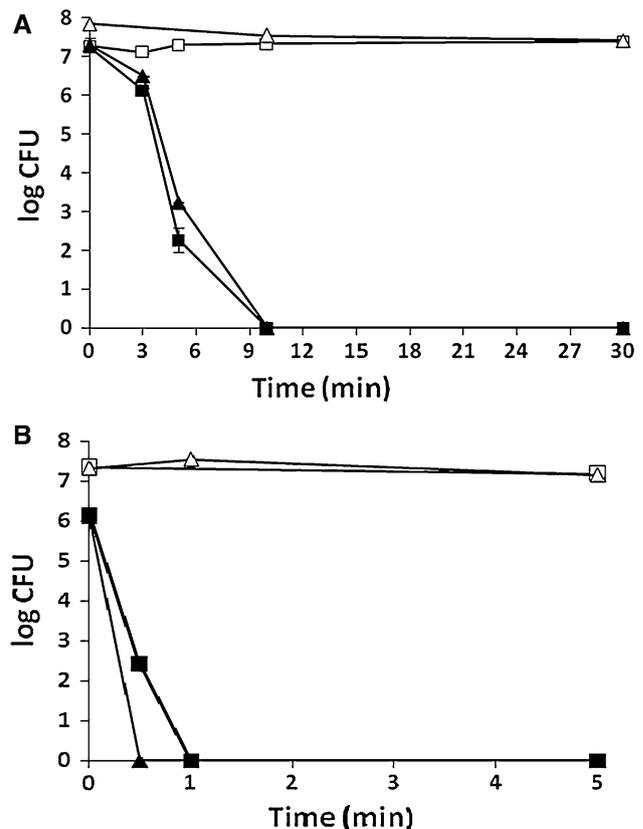
**Fig. 1** Survival of *C. sakazakii* BAA-894 *E. sakazakii* MZ0685 suspended in TSB on 99.9% copper (filled square) and stainless steel (open square) in moist environmental conditions (a) and quick air drying (b). Survival rates are also shown after 33 days desiccation in TSB, on 99.9% copper (filled triangle) and stainless steel (open triangle)
