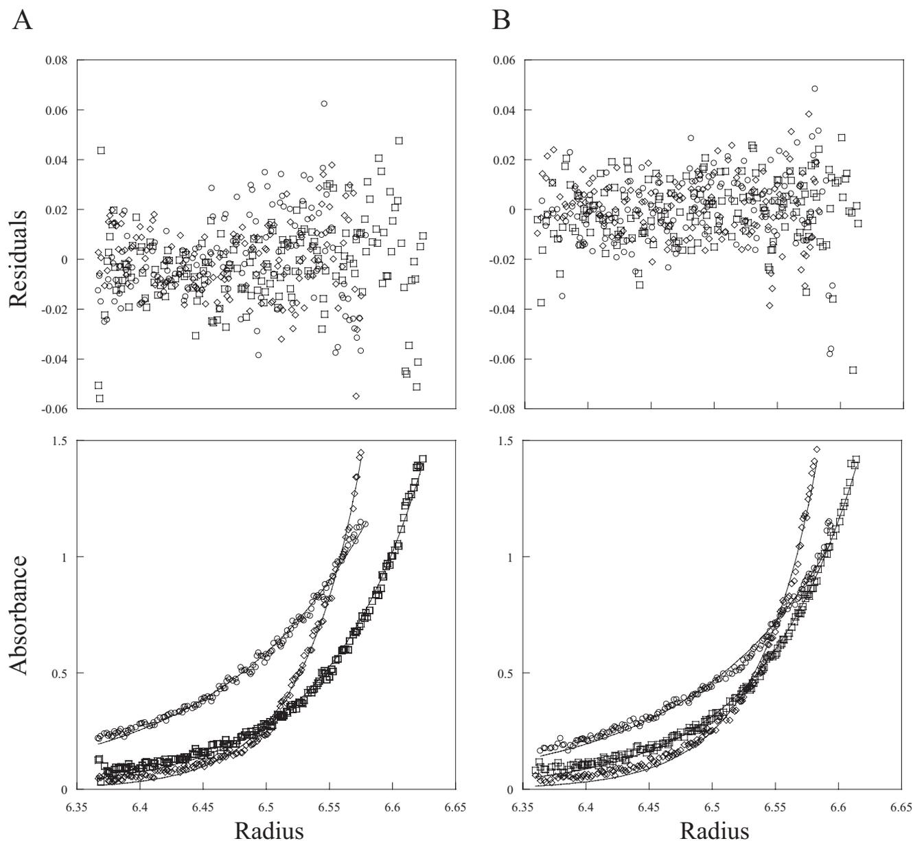
**FIGURE 4. Sedimentation equilibrium analysis of apo-CusB (A) and CusB-Ag(I) (B).** Bottom panels show data points and curve fits for protein at a concentration of  $\sim 9 \mu\text{M}$  ( $A_{280} = 0.43$ ) at three different speeds of 15,000 ( $\circ$ ), 20,000 ( $\square$ ), and 25,000 ( $\diamond$ ) rpm with scans at 280 nm. Top panels show the residuals when subtracting the calculated values from the measured points.
