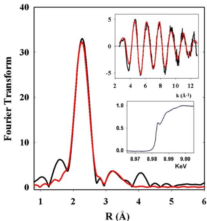
FIGURE 2. EXAFS data for CusB-Cu(I). Experimental (black) and simulated (red) Fourier transforms and EXAFS (top inset) for CusB-Cu(I). X-ray absorption edge intensity of 8983 eV is diagnostic of 3-coordinate geometry (bottom inset).
