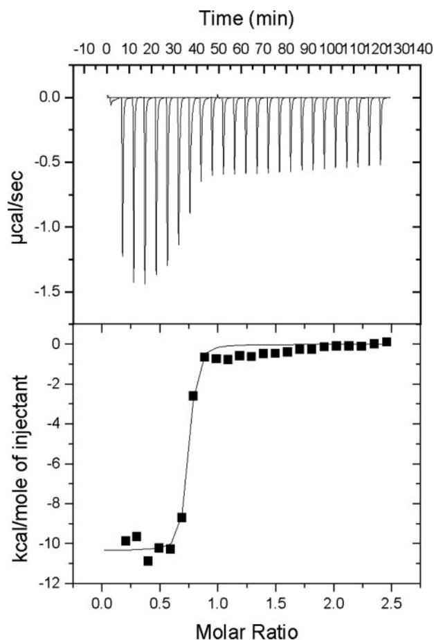
FIGURE 1. ITC data for titration of 22  $\mu\text{M}$  CusB with 300  $\mu\text{M}$   $\text{AgNO}_3$  at 25  $^\circ\text{C}$ . Both solutions were made in 50 mM cacodylate (pH 7.0). Top, raw data. Bottom, plot of integrated heats versus  $\text{Ag(I)}/\text{CusB}$  ratio. The solid line represents the best fit for a one-site binding model.
