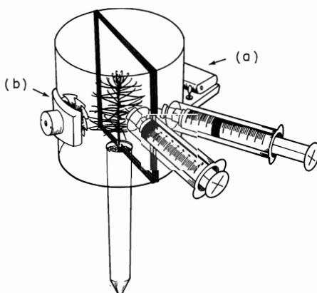
Fig. 1. Hand-held plexiglass photosynthesis chamber for measuring *in situ* CO<sub>2</sub> fixation rates of Douglas-fir seedlings. (a) Battery-operated, (b) fan circulates air during fixation periods.
