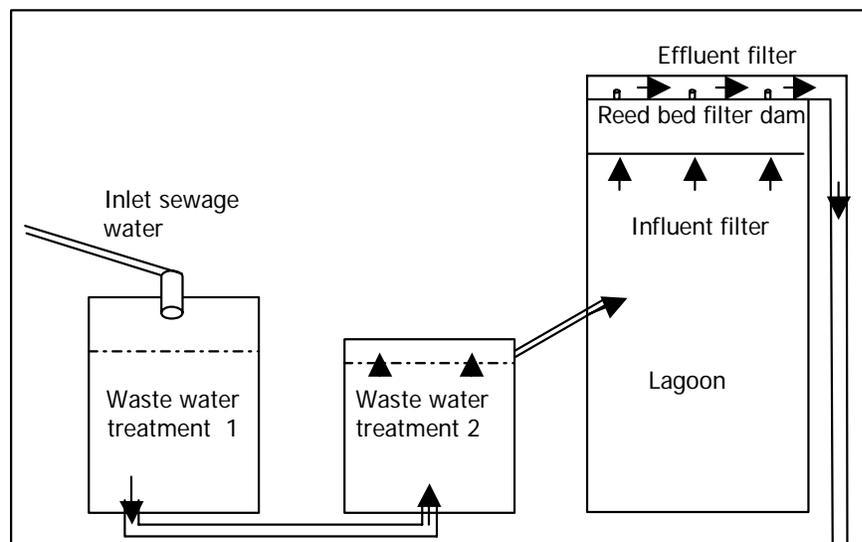
**Figure 1.** Schematic outline of a typical municipal waste water treatment lagoon, in this case equipped with a phytoremediation filter.
