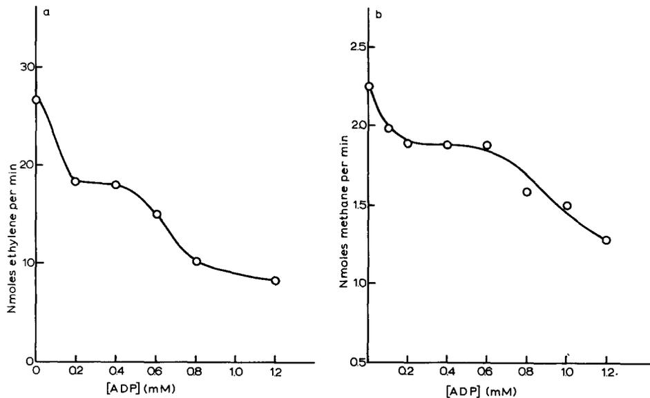
Fig. 4. Inhibition of acetylene (a) and  $\text{CN}^-$  (b) reduction by ADP with constant ATP (10 mM). (a) 0.8 mg protein *ex* DEAE-cellulose (b) 0.4 mg *ex* DEAE-cellulose: ATP/MgCl<sub>2</sub> = 0.5. Agreement between duplicate analysis was good; S.D. = 0.9 nmole acetylene and 0.02 nmole methane.
