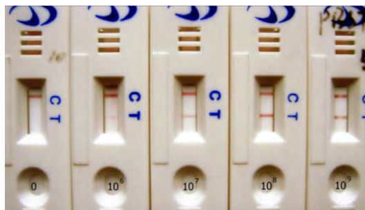
Fig. 2 Rapid immunogold quicktests for 1N ( Pseudomonas fluorescens ), a component of BioGro used in rice production
