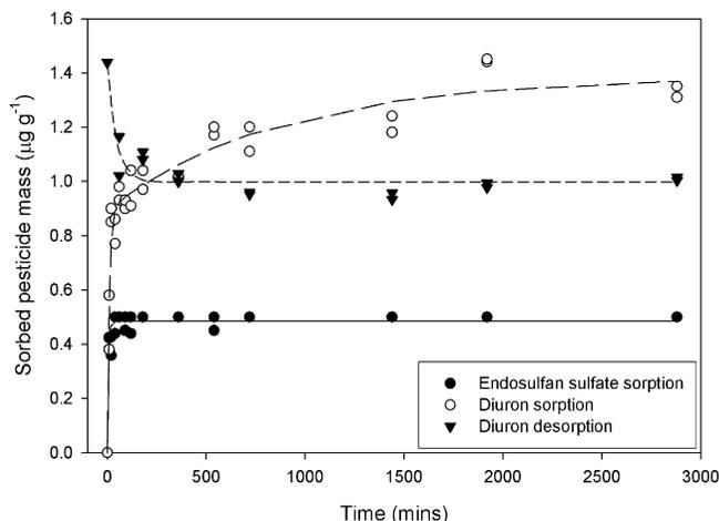
**Figure 1.** Endosulfan sulfate and diuron sorption and desorption kinetics showing observed and fitted results for sorbed mass of each pesticide ( $\mu\text{g g}^{-1}$ ) against time (min). (Endosulfan sulfate sorption, adj.  $R^2 = 0.96$ ; diuron sorption, adj.  $R^2 = 0.96$ ; and diuron desorption, adj.  $R^2 = 0.90$ ).
