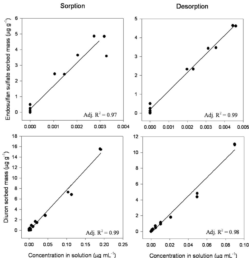
**Figure 2.** Sorption and desorption isotherms for endosulfan sulfate (top left and top right, respectively) and diuron (bottom left and bottom right, respectively) depicting observed and fitted results of sorbed pesticide mass ( $\mu\text{g g}^{-1}$ ) against pesticide concentration in solution ( $\mu\text{g mL}^{-1}$ ) and their respective coefficients of determination (adj.  $R^2$ ).
