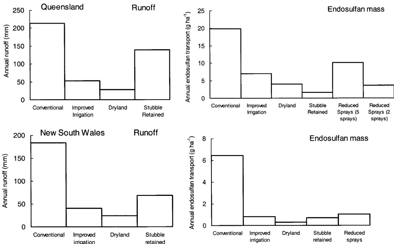
Fig. 4. Predicted average annual runoff and endosulfan transport from the two sites. Runoff from the Reduced Sprays scenario is the same as Conventional.
