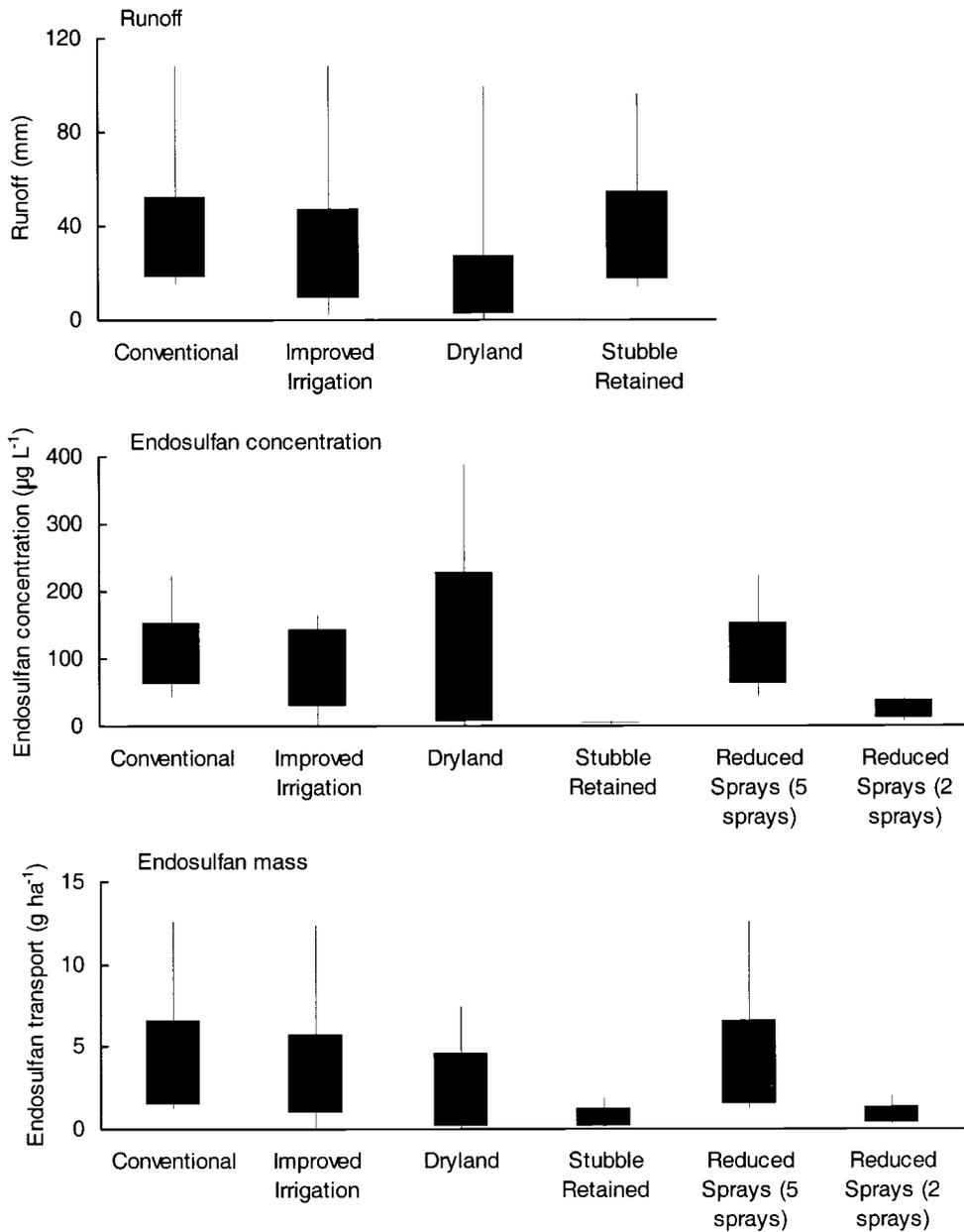
Fig. 6. Daily runoff, endosulfan concentration, and mass predicted in large events at the Queensland site, calculated using an annual series. Top and bottom of the thin bars are the 1:30 and 1:1 year probabilities, top and bottom of the thick bars are the 1:10 and 4:5 year probabilities, respectively. Runoff in the Reduced Sprays scenario is the same as Conventional. Note: Data for runoff, concentration, and mass are calculated independently, and may not be from the same event.
