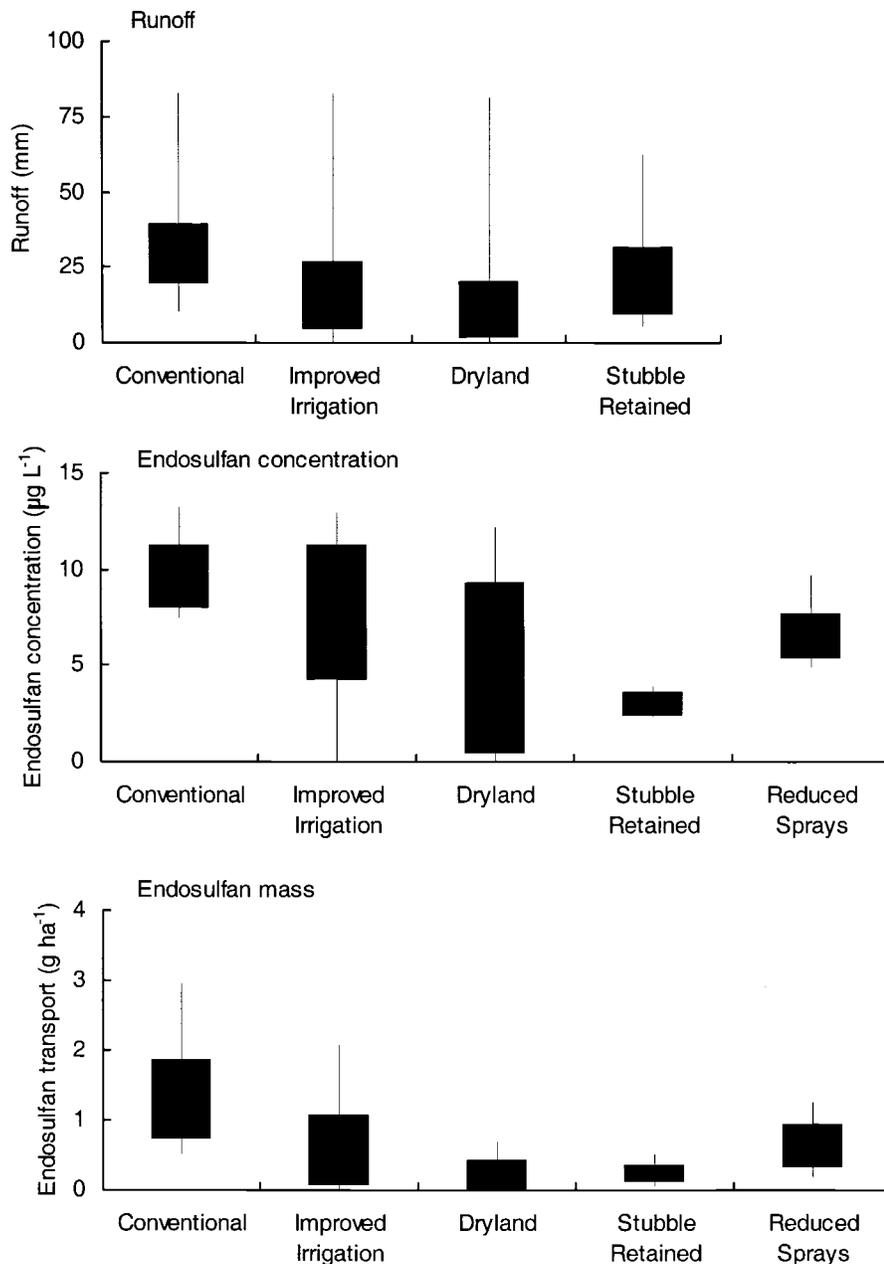
Fig. 7. Daily endosulfan mass and concentration predicted in runoff from large events at the New South Wales site. Top and bottom of the thin bars are the 1:30 and 1:1 year probabilities, top and bottom of the thick bars are the 1:10 and 4:5 year probabilities, respectively. Runoff in the Reduced Sprays scenario is the same as Conventional.
