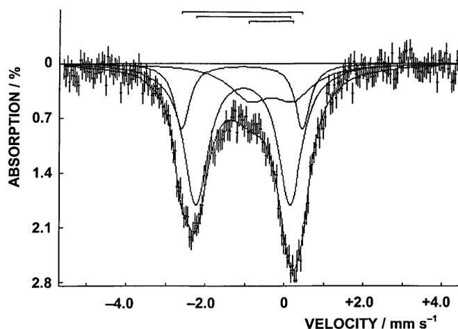
**Fig. 2** Emission Mössbauer spectrum of cation-free glutamine synthetase from *Azospirillum brasilense* Sp245 activated by  $^{57}\text{Co}^{2+}$  (frozen solution;  $T=80\text{ K}$ )
