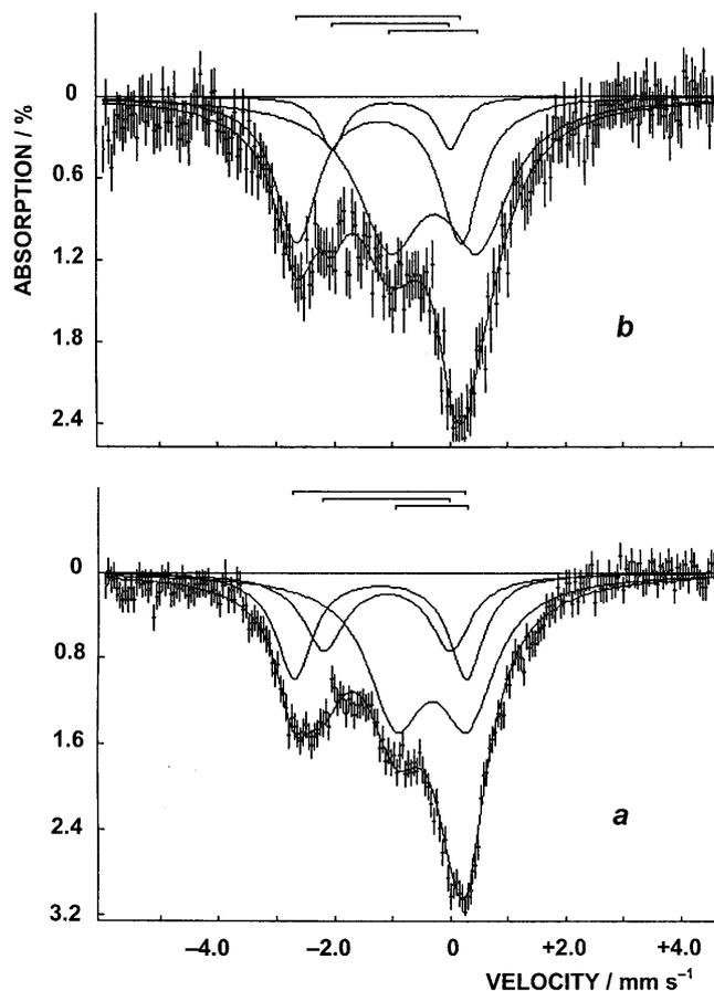
**Fig. 1** Emission Mössbauer spectra of *Azospirillum brasilense* Sp245 living cells frozen (a) 2 min and (b) 1 h after incubation with trace <sup>57</sup>CoCl<sub>2</sub> (dried; T=80 K)
