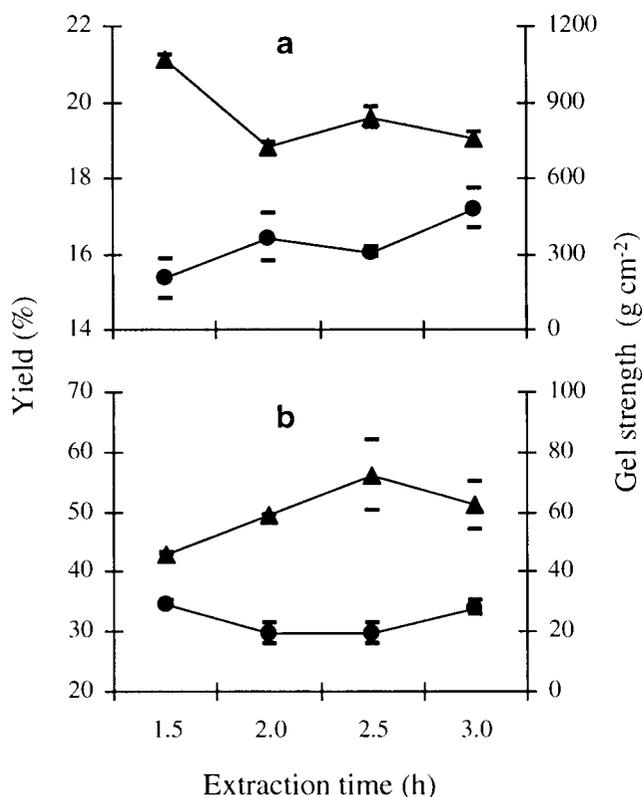
**Fig. 2** Agar yield (●) and gel strength of 1.5% agar (▲) from *Gracilaria vermiculophylla* with different extraction times. **a** Alkali treated agar, **b** native agar. Bars represent standard error (±SE)
