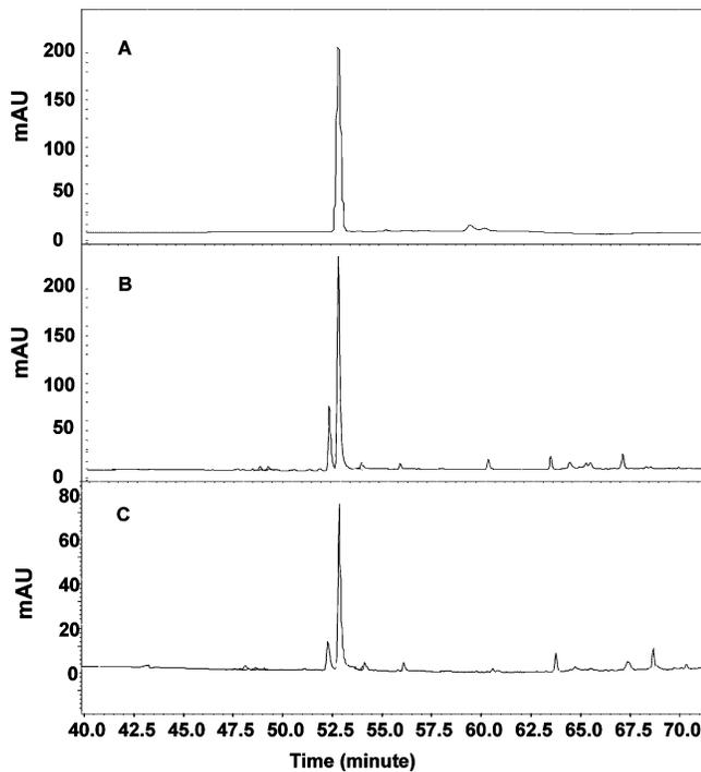
**Figure 3.** HPLC chromatograms of the blond and red grapefruits in dimethyl sulfoxide (DMSO) fractions: (A) naringin, 52.75 min; (B) blond grapefruit, 52.75 min; (C) red grapefruit, blond grapefruit, 52.74 min. The major peak is due to naringin, the dominant phenolic compound in grapefruits. See text for detailed HPLC conditions.
