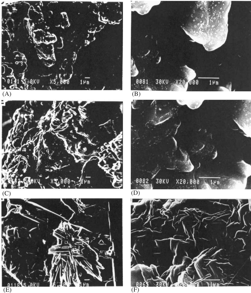
**Figure 2.** Microstructure of isopropanol-soluble proteins from (A) and (B) amaranth, (C) and (D) soybean, and (E) and (F) maize (prolamins). A, C and E, magnification  $\times 5000$ ; B, D and F, magnification  $\times 20,000$ .
