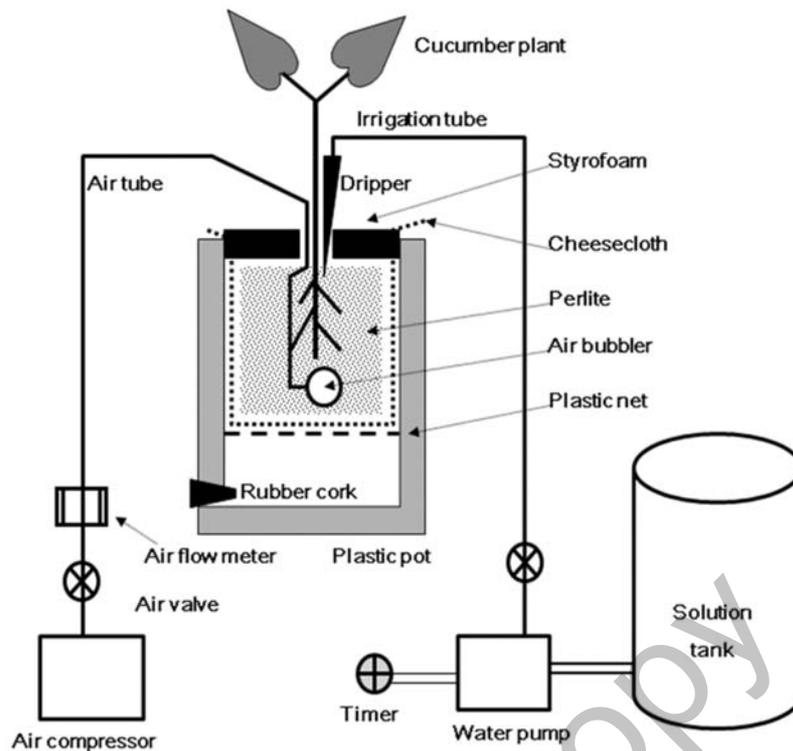
Fig. 1. Schematic diagram of the experimental system for forced aeration treatment.
