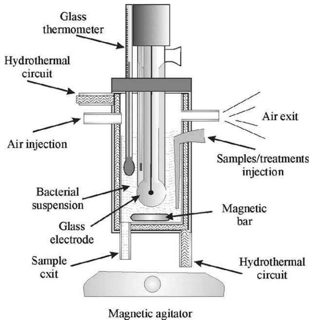
Fig. 1. Bioreactor used to monitor hydrogen activity: open system with glass electrode and controlled air flux, agitation and temperature.
