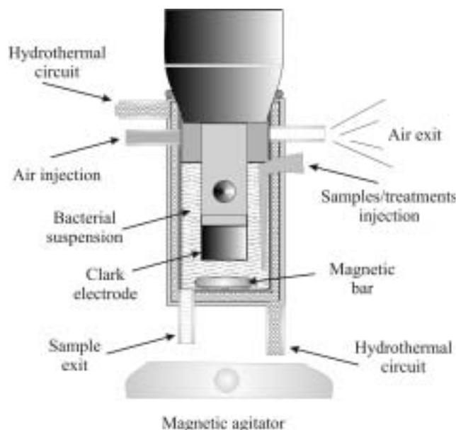
Figure 1. Bioreactor used to monitor dissolved oxygen activity: open system with Clark's electrode and controlled air flux, agitation and temperature.
