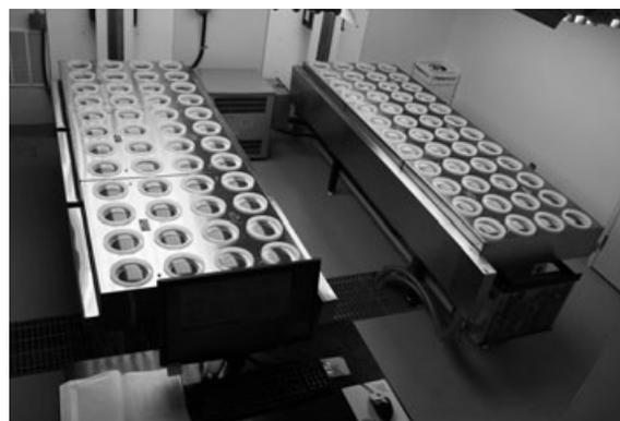
Figure 2 A thermogradient plate unit with 96 independently temperature-controlled wells.
