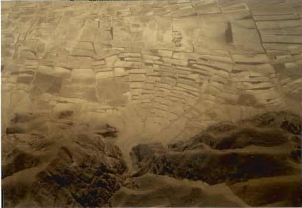
Figure 5. Examples of small dikes used to capture water and sediment runoff from the mountains.
