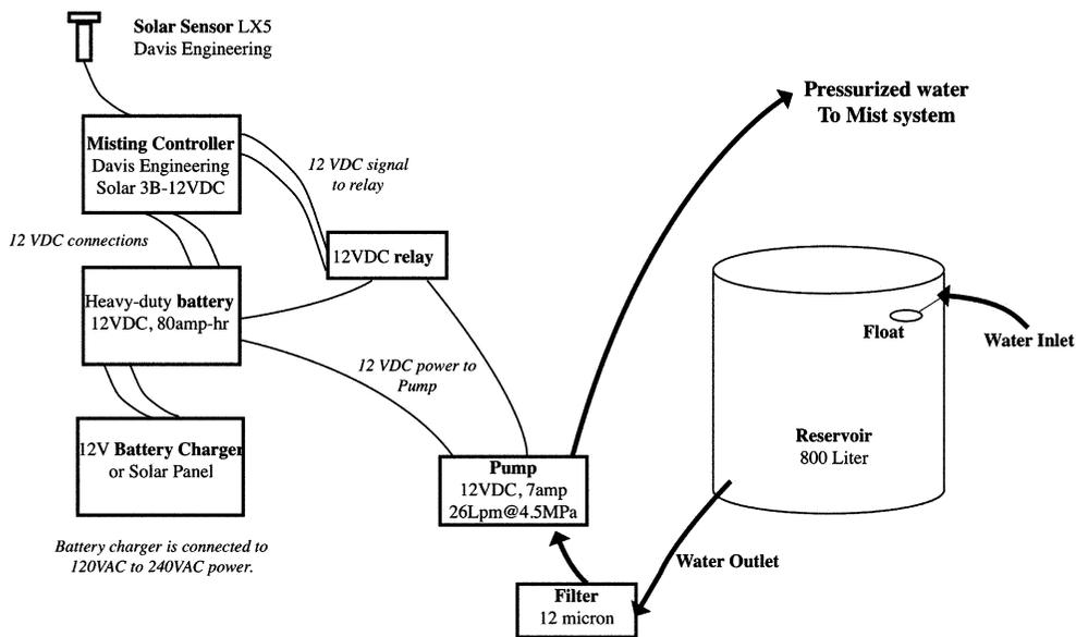
**Fig. 1** Schematic diagram for a light intensity controlled, high-pressure mist system with DC backup power for rooting cuttings
