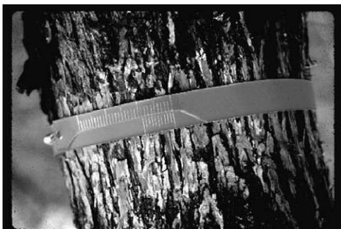
Fig. 1. Painted aluminum dendrometer band permanently attached to a *Prosopis* tree trunk after the loose bark was scraped off.
