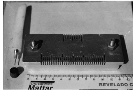
Fig. 2. Improved tool for making dendrometer bands. The stylus used to inscribe the bands is to the left. Dimensions are as noted in the text.
