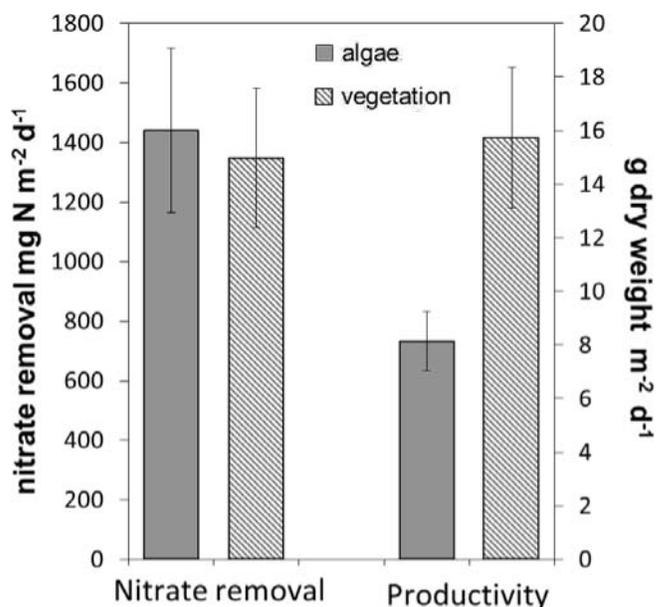
**Fig. 3.** Differences in mean nitrate removal rate and productivity in the selectively harvested algal-dominated module compared to the unselectively harvested module containing a mixed vegetation of aquatic macrophytes and algae; 18 May 2008 to 19 August 2008. Error bars indicate 95% confidence intervals ( $n = 30$ ).
