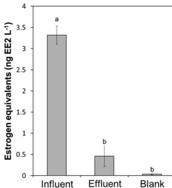
**Fig. 6.** EE2-equivalence of water from influent and effluent of the unselectively harvested module and the water-only blank treatment. Significance was determined by a Tukey-Kramer MSD test. Means ( $\pm$  SE) having the same letter are not significantly different from each other ( $n = 4$ ).
