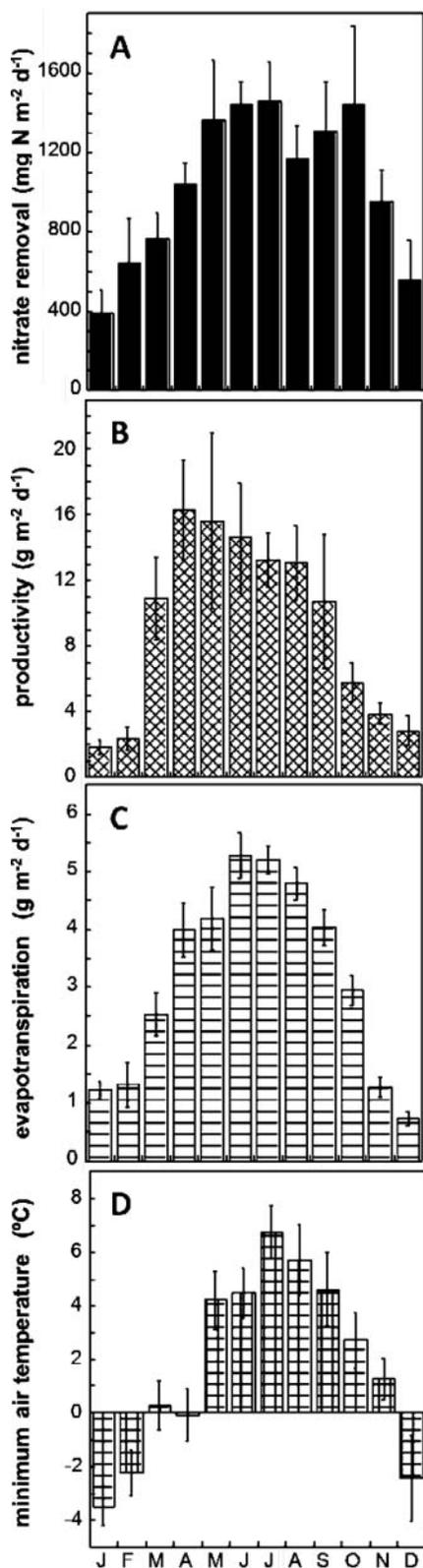
**Fig. 2.** Monthly means of (A) nitrate removal rate, (B) productivity, (C) evapotranspiration, and (D) minimum air temperature. Error bars indicate 95% confidence intervals; all data are from unselectively harvested modules from 13 May 2008 to 1 December 2009 (A:  $n = 95$ ; B, C, D:  $n = 279$ ).
