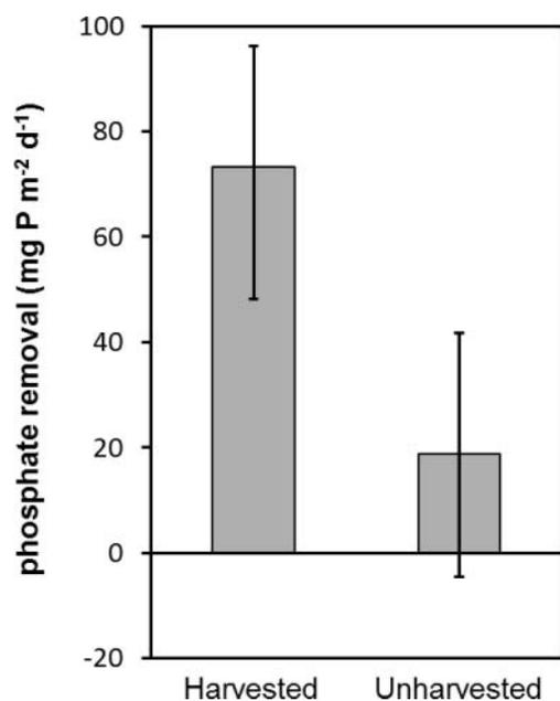
**Fig. 4.** Phosphate removal rates of harvested and unharvested modules; 3 November 2009 to 19 October 2010. Error bars indicate 95% confidence intervals ( $n = 48$ ).
