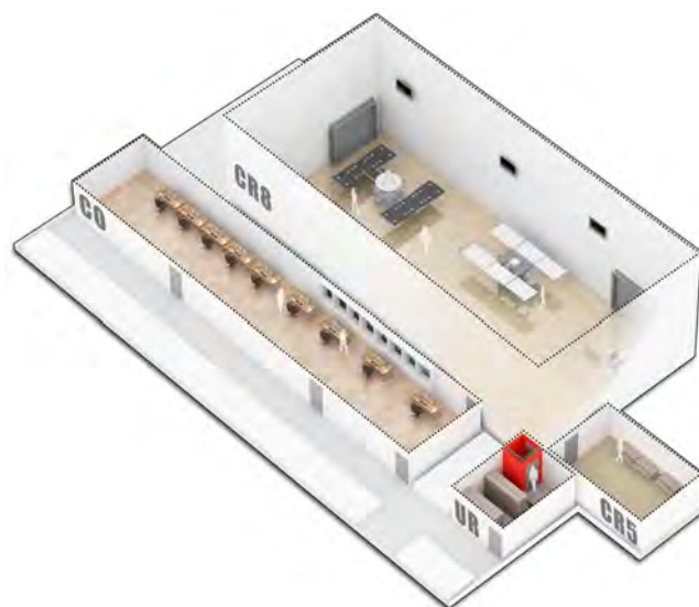
Figure 1 | Illustration of the integration center at Airbus Defence and Space GmbH in Friedrichshafen, Germany. Sampled rooms were designated as follows: UR – changing room, CO – checkout room, CR8 – ISO 8 cleanroom, CR5 – ISO 5 cleanroom. Proportions reflect actual dimensions. Interior decorations were abstracted and do not mirror real arrangement.
