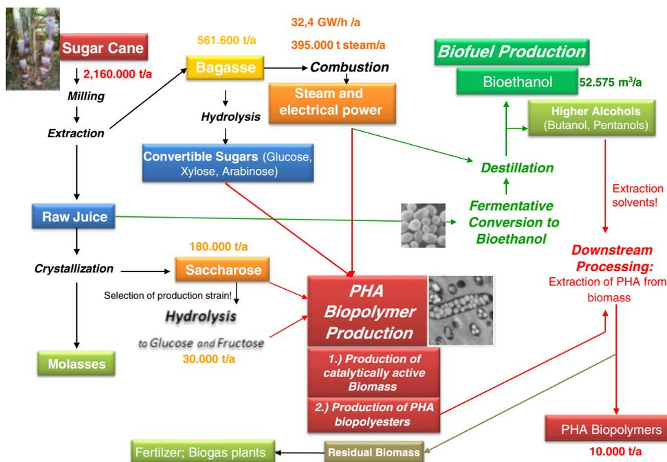
**Figure 7.** Embedding of PHA production into the sugarcane and bioethanol industry at PHBISA, Brazil.
