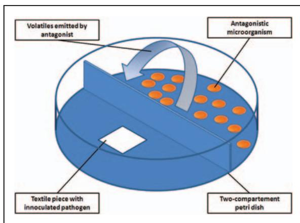
**Figure 4.** Two-compartment petri dish showing a dual-culture assay for the detection of volatile antimicrobials, produced by bacteria. The textile pieces were inoculated with pathogenic microorganisms. Co-incubation with plant-associated bacteria allowed VOCs to diffuse into the chamber containing the pathogen-inoculated textile piece.
