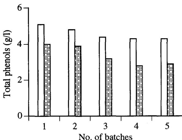
Fig. 2. Phenol concentration of OMW-based media as affected by immobilized *A. niger*. Open symbols, OMW; shaded symbols, OMW+RP.
